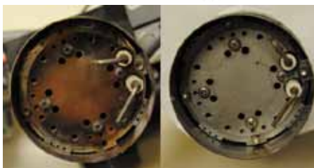
Example of non-functioning & functioning burners.
