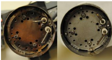
Example of non-functioning & functioning burners.
