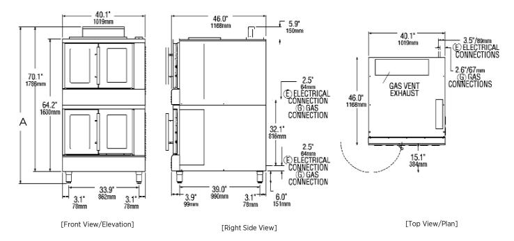
INSTALLATION REQUIREMENTS: Two 120V 1-Phase, 50/60 Hz electrical connections [Cords & Plugs supplied]
