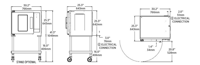
**INSTALLATION REQUIREMENTS:** Single 208V/240V, 1- or 3-Phase; optional 480V, 3- phase electrical connection only on ECOH-AP model [Power connection from rear]
