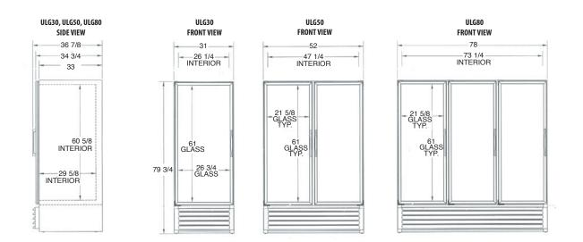
Cabinet designed for optimum performance in air-conditioned area at 70°F to 75°F ambient temperature and 50% to 55% relative humidity.
